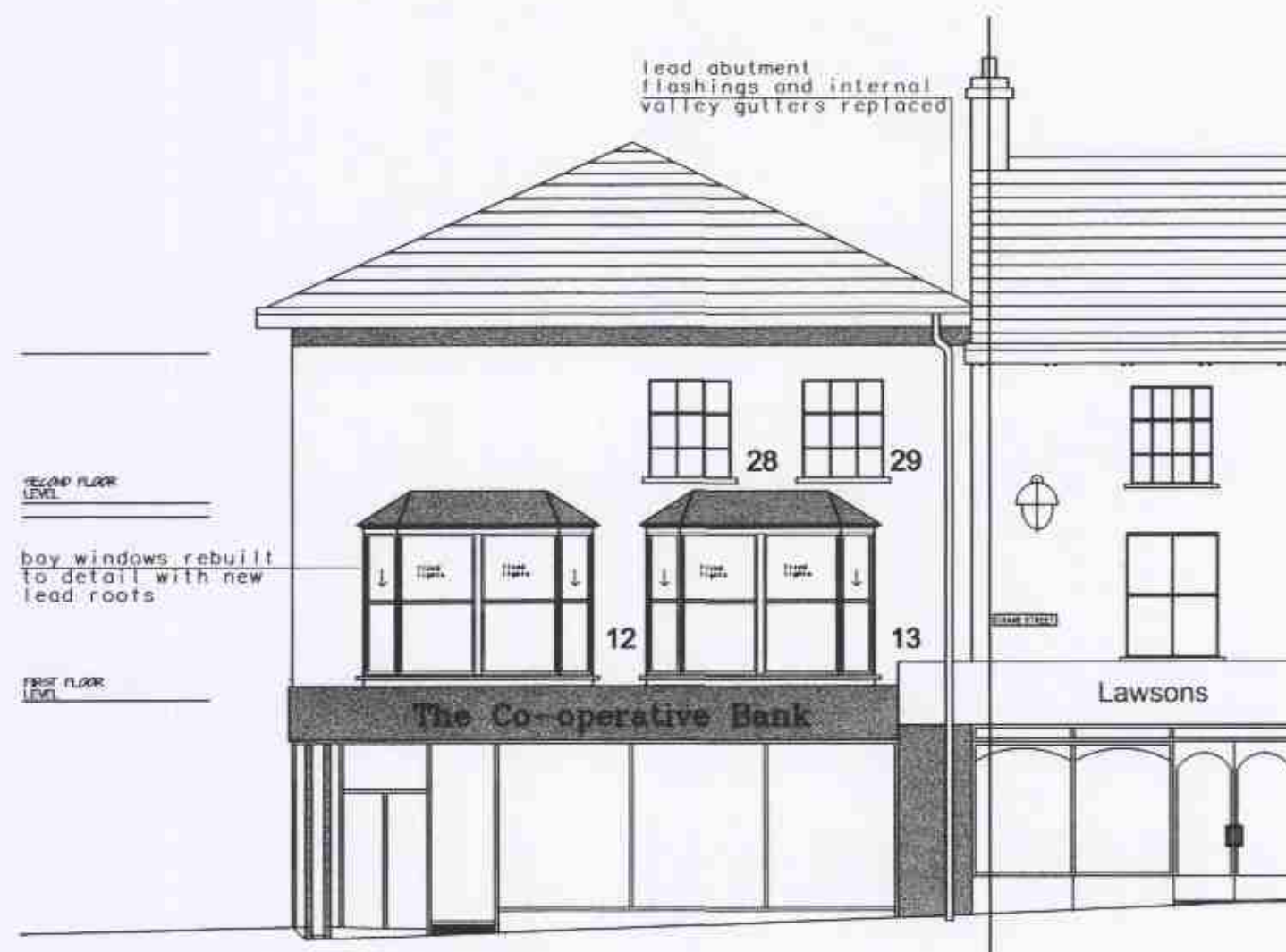
FRONT ELEVATION TO CRANE STREET PROPOSED
